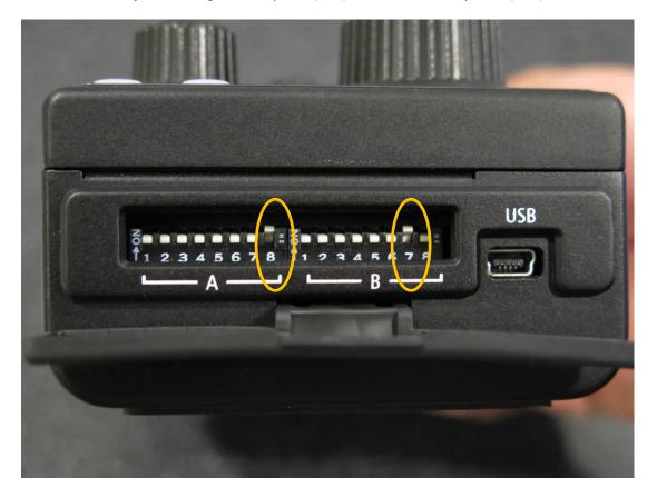
panel at base of controller. Ensure controller disconnected before making adjustments
